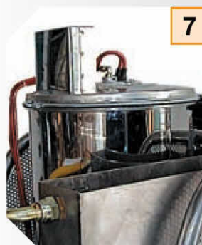
STAINLESS STEEL Industrial heating system and water feed tank made of stainless steel
