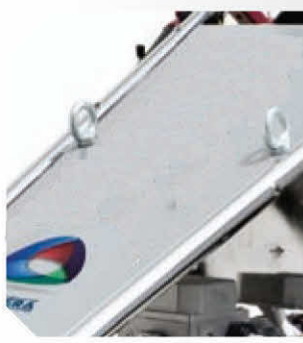
EYE BOLTS allows the machine to be moved easily in the yard.
